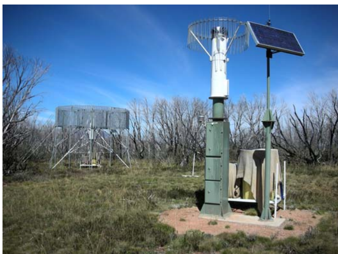
Figure 1.2 Grey Hill site, showing a pedestal (foreground) and tripod (background) pluviometer with and without wind fences (March 2007)
