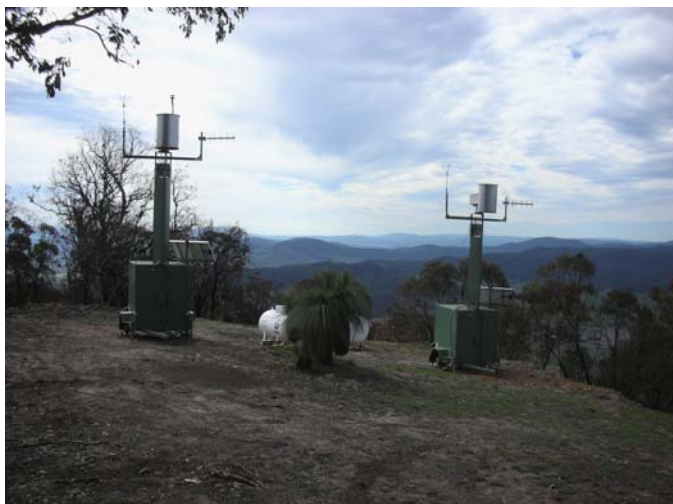
Figure 1.1 Indi generator site, showing LPG tanks and trailer-based silver and indium generators (March 2007)
